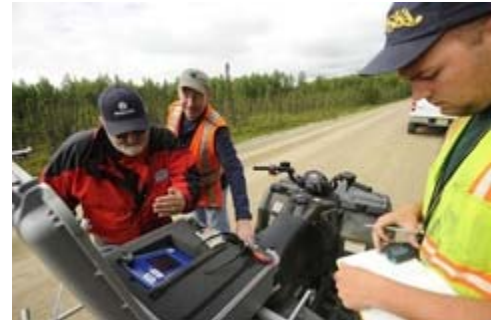
enlarge MARC LESTER / Anchorage Daily News Ron Harvey, left, of Freedom Industries in Palmer, looks at an ATV-mounted instrument for measuring dust kicked up on an unpaved road near Knik Goose Bay Road about 12 miles southwest of Wasilla on July 1, 2010. Dave Barnes, center, and Travis Eckhoff of UAF took measurements to gather information about a Freedom Industries dust control application being tested there.
