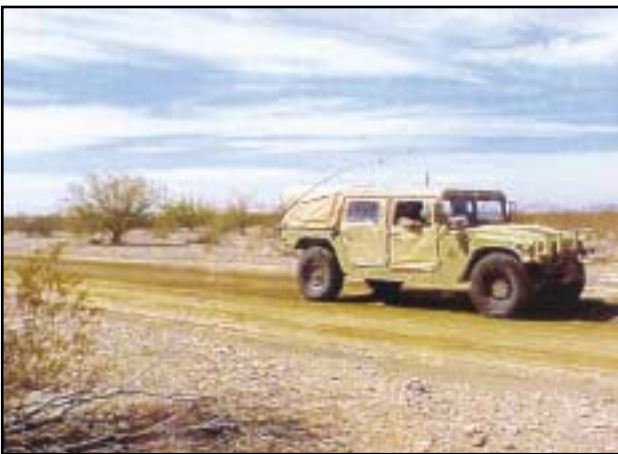
Photo 1: Humvee generates little to no dust as it travels along the EnviroKleen®-treated Main Supply Route.
