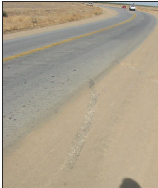
Photo 6 Hard, Straight Acceleration on Soil Sement®
