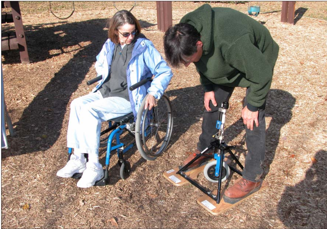
Figure 9—Measurement of accessibility with rotational penetrometer.
