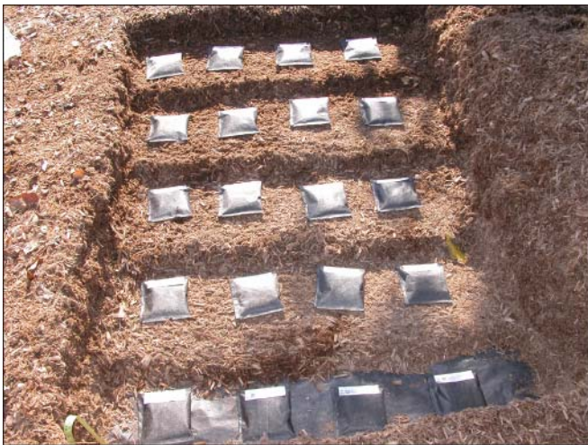
Figure 11—Biodeterioration samples on EWF surface.
