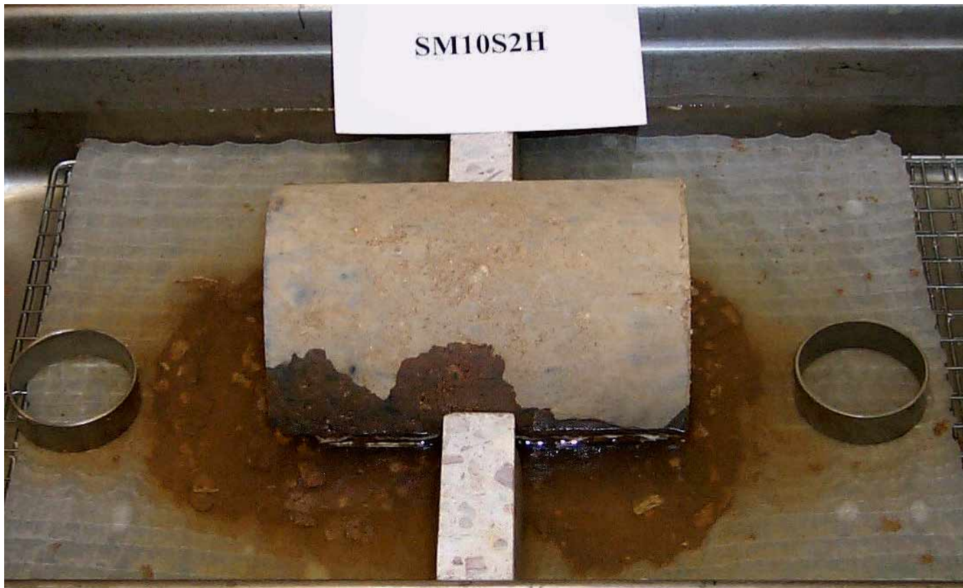
FIGURE 3 Enzyme 1 stabilizer during the 15-minutes soaking period of the wet test
