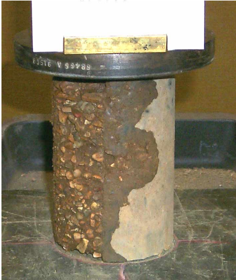
FIGURE 4 Enzyme 1 stabilizer after the wet test
