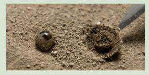
A side by side comparison: The high surface tension of a water droplet (left) prevents it from penetrating and coating dust particles. Midwest's CDS-8040 foam agent (right), which has low surface tension quickly blankets dust particles so they do not become airborne.
