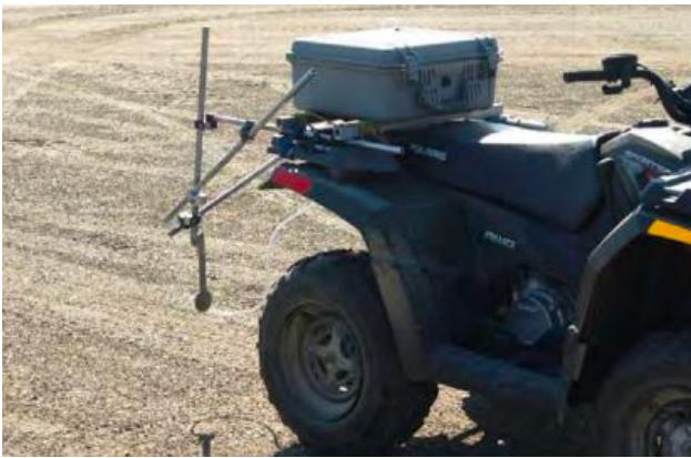
EVALUATING DUST PALLIATIVE PERFORMANCE AND LONGEVITY USING THE UAF-DUSTM FIGURE 1: UAF-DUSTM mounted on an ATV for data collection
