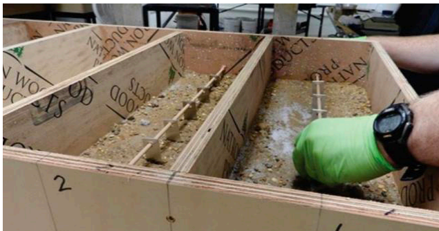
Metal Coupon Placement
