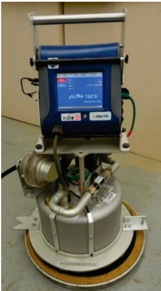
ERDC/GSL TR-21-31 FIGURE 12: PI-SWERL Laboratory Test Setup
