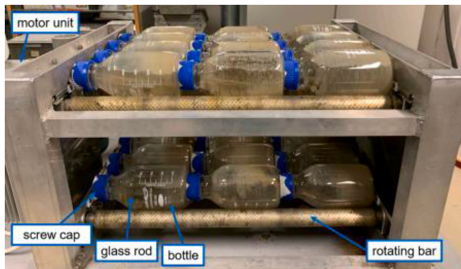
TRANSPORTATION GEOTECHNICS FIGURE 6: Rolling machine setup with test bottles
