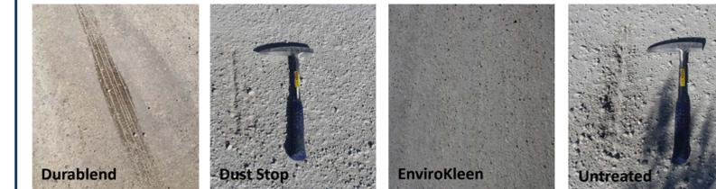
Figure 2. Representative photos of treated road surfaces.
