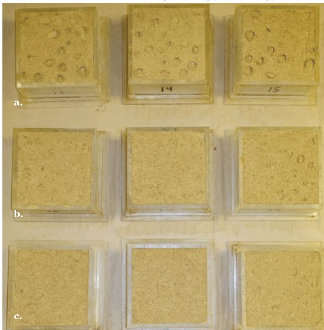
Figure A22. Test specimens treated with X-Hesion Pro, after air impingement testing, at application rates of (a) 0.4 gsy, (b) 0.8 gsy, and (c) 1.2 gsy.
