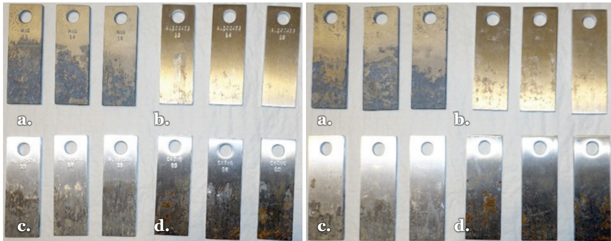
Figure A61. Metal coupons after 90 days in soil treated with GRT 9000: (left) fronts and (right) backs. Metals are (a) magnesium, (b) aluminum T3, (c) aluminum T6, and (d) steel.
