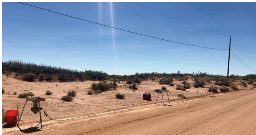
Figure 40. Layout of stationary dust collectors.
