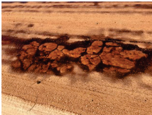
(e) Pooling of product after spraying on Item 4.
