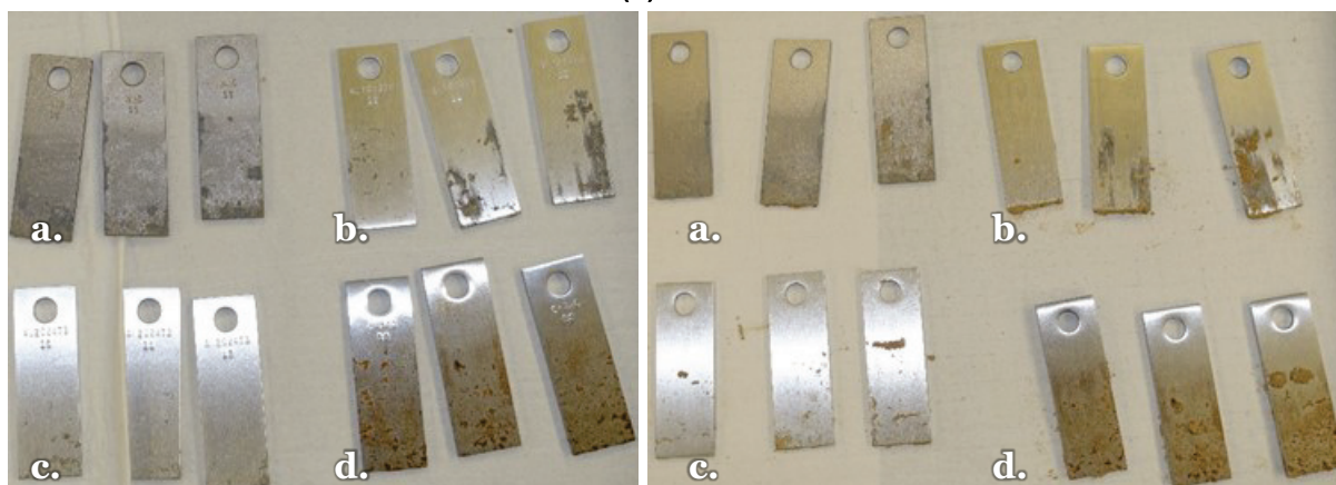
Figure A56. Metal coupons after 30 days in soil treated with Triple Tac: (left) fronts and (right) backs. Metals are (a) magnesium, (b) aluminum T3, (c) aluminum T6, and (d) steel.
