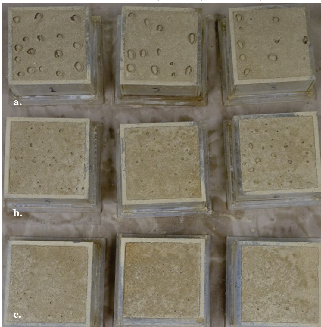
Figure A18. Test specimens treated with GRT 9000, after air impingement testing, at application rates of (a) 0.4 gsy, (b) 0.8 gsy, and (c) 1.2 gsy.
