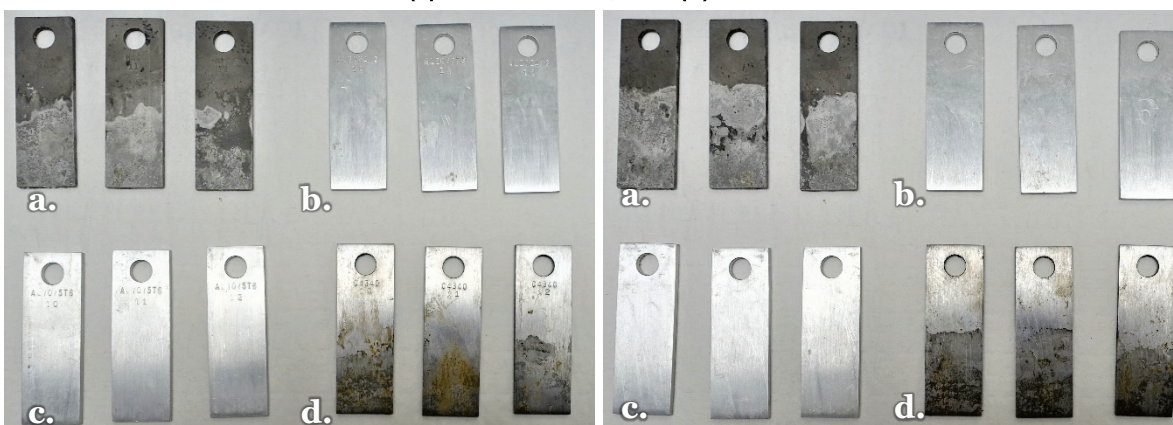
Figure A90. Metal coupons after 120 days in soil treated with BioSoyl Plus: (left) fronts and (right) backs. Metals are (a) magnesium, (b) aluminum T3, (c) aluminum T6, and (d) steel.
