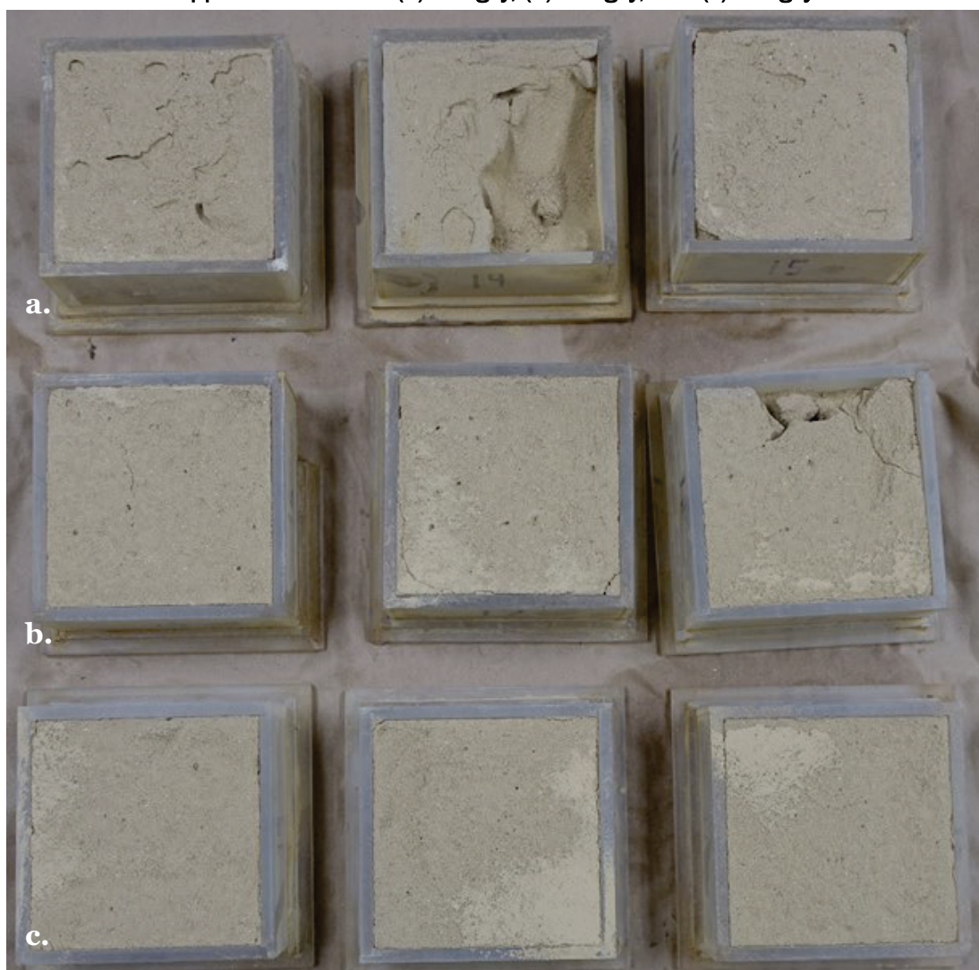
Figure A2. Test specimens treated with water, after air impingement testing, at application rates of (a) 0.4 gsy, (b) 0.8 gsy, and (c) 1.2 gsy.
