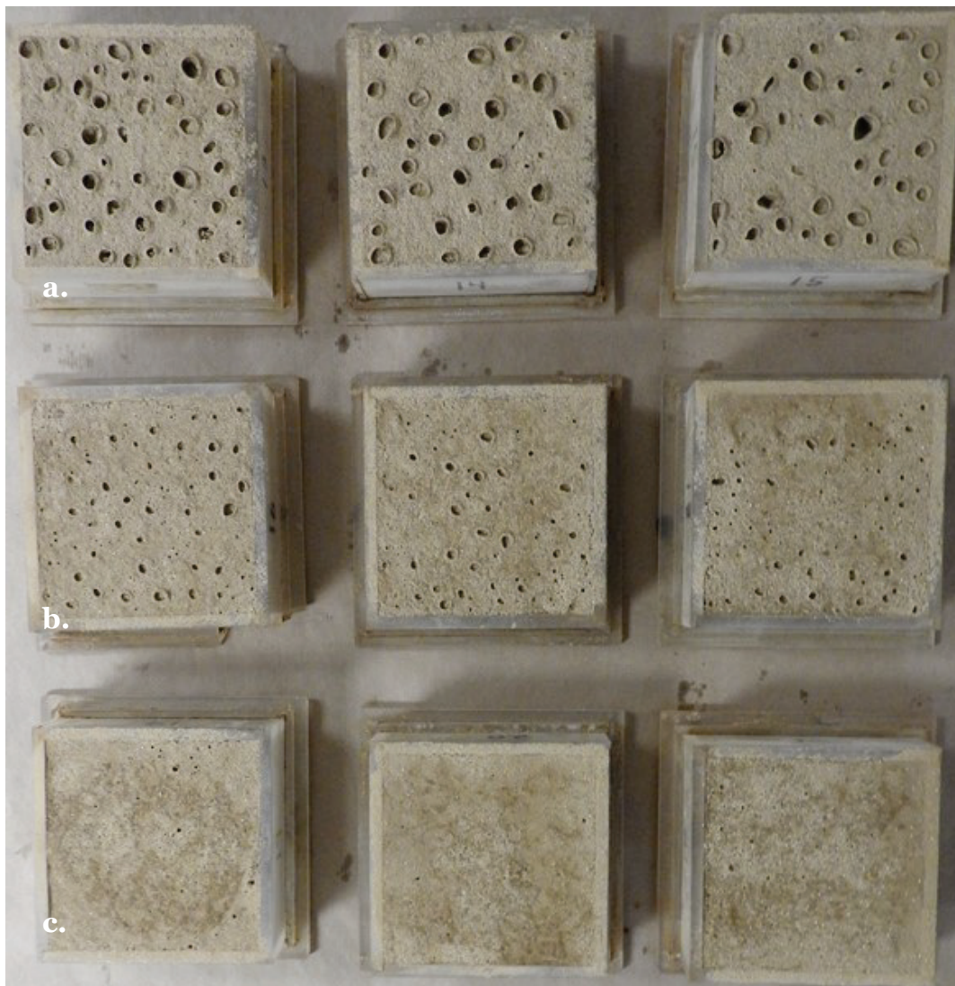
Figure A12. Test specimens treated with DustPly Plus C, after air impingement testing, at application rates of (a) 0.4 gsy, (b) 0.8 gsy, and (c) 1.2 gsy.
