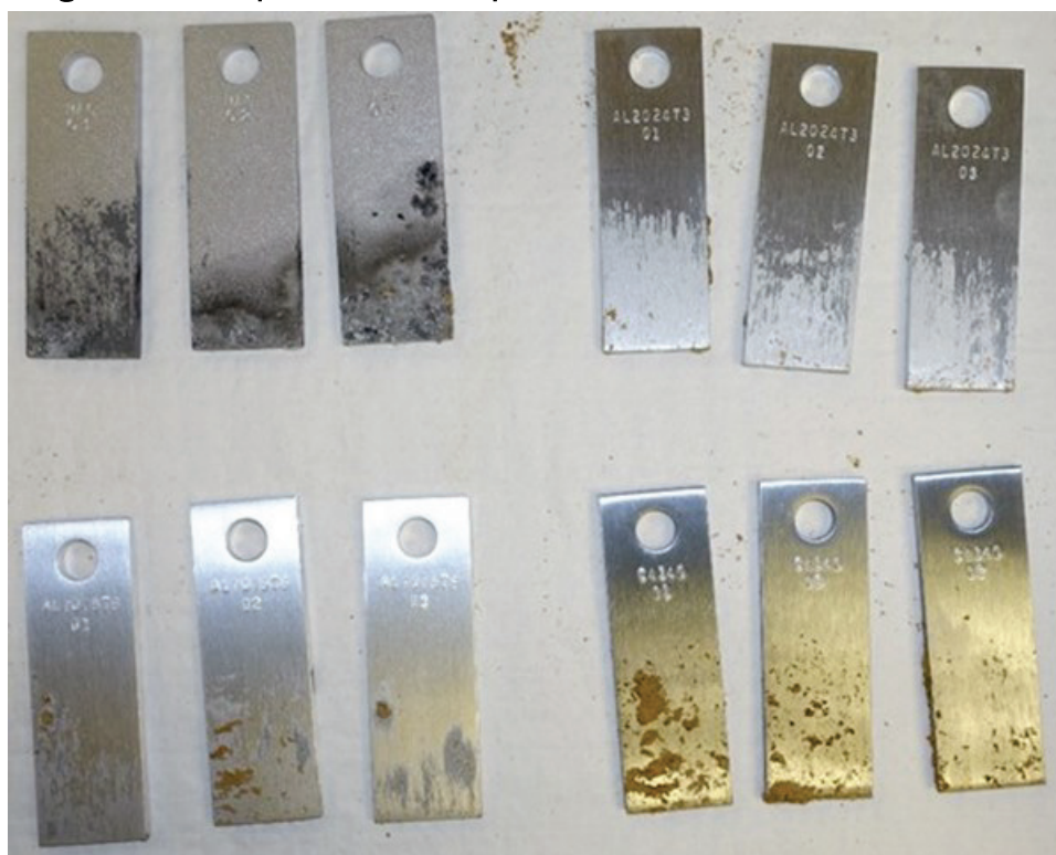
Figure 19. Examples of metal coupons after removal from the treated soil.
