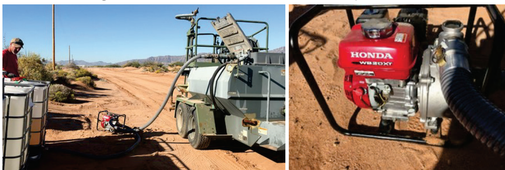
Figure 33. Pump used to add palliatives to hydroseeder.
