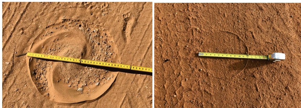
Figure 46. Example of pre-application (left) and post-application (right) of the palliative before the PI-SWERL test is applied.
