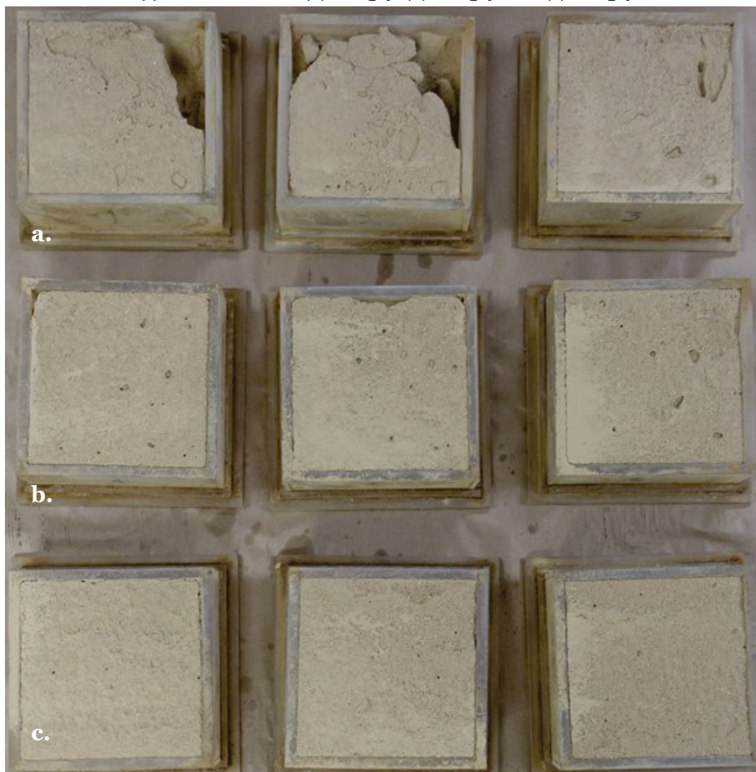
Figure A16. Test specimens treated with Triple Tac, after air impingement testing, at application rates of (a) 0.4 gsy, (b) 0.8 gsy, and (c) 1.2 gsy.
