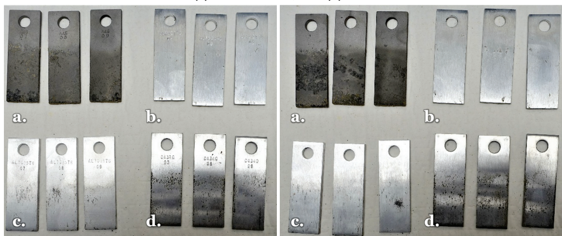
Figure A74. Metal coupons after 120 days in soil treated with SandTec 9006: (left) fronts and (right) backs. Metals are (a) magnesium, (b) aluminum T3, (c) aluminum T6, and (d) steel.
