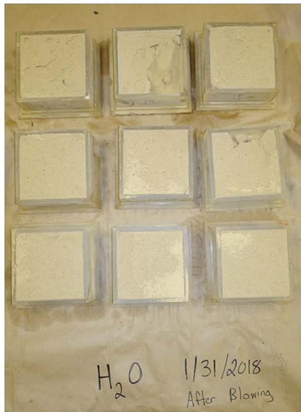
Figure 6. Example soil samples after wind chamber test with water as the dust agent.
