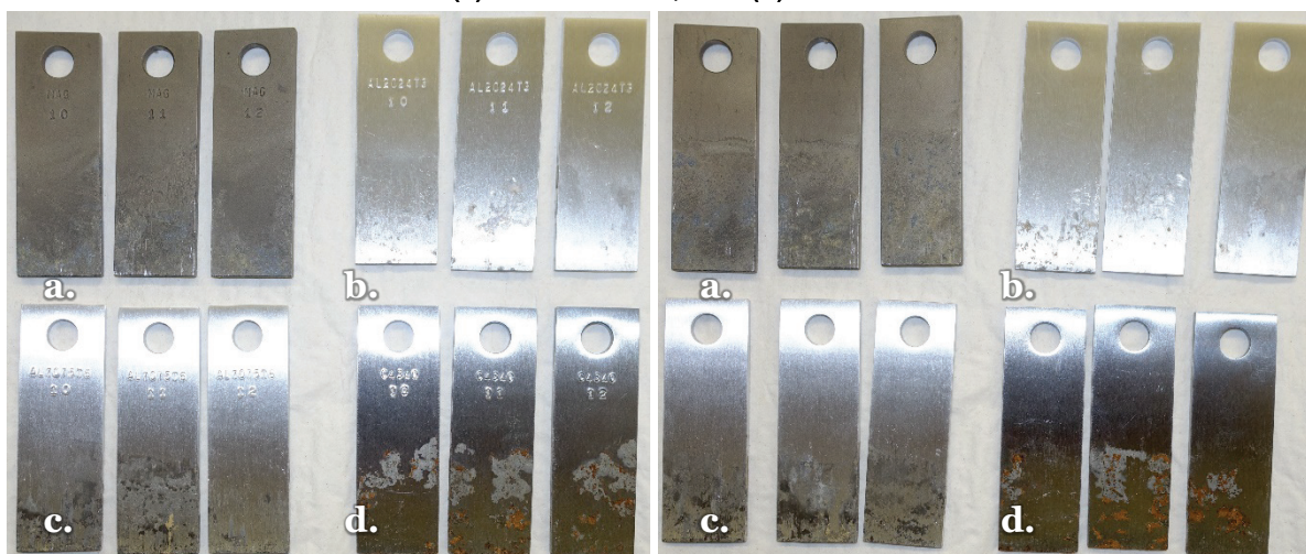
Figure A42. Metal coupons after 120 days in soil treated with DustPly Plus C: (left) fronts and (right) backs. Metals are (a) magnesium, (b) aluminum T3, (c) aluminum T6, and (d) steel.
