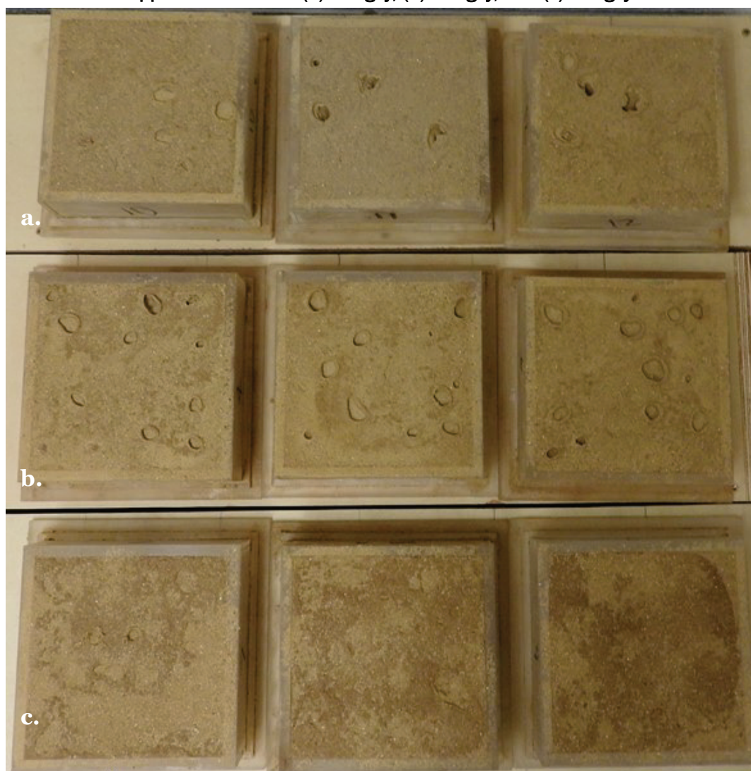
Figure A4. Test specimens treated with Soiltac, after air impingement testing, at application rates of (a) 0.4 gsy, (b) 0.8 gsy, and (c) 1.2 gsy.
