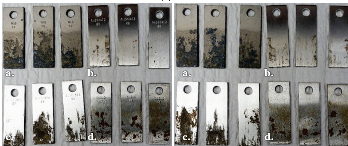
Figure A29. Metal coupons after 30 days in soil treated with water: (left) fronts and (right) backs. Metals are (a) magnesium, (b) aluminum T3, (c) aluminum T6, and (d) steel.
