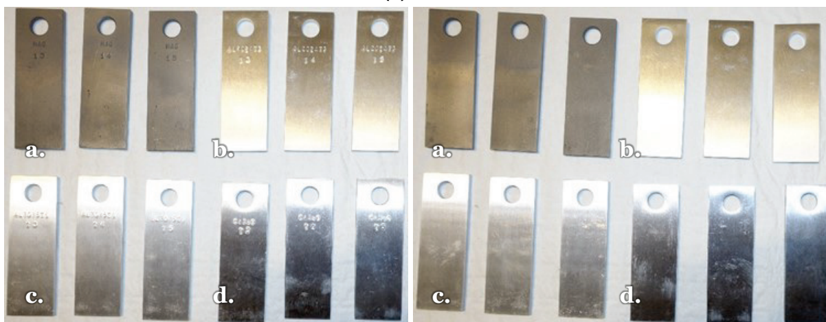
Figure A47. Metal coupons after 360 days in soil treated with EK35: (left) fronts and (right) backs. Metals are (a) magnesium, (b) aluminum T3, (c) aluminum T6, and (d) steel.
