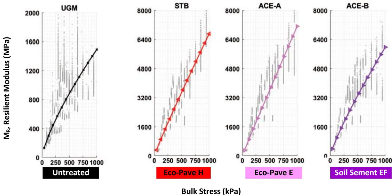
Figure 3: Comparison of resilient modulus between untreated aggregate (left) and NaturalPave treated aggregate.
