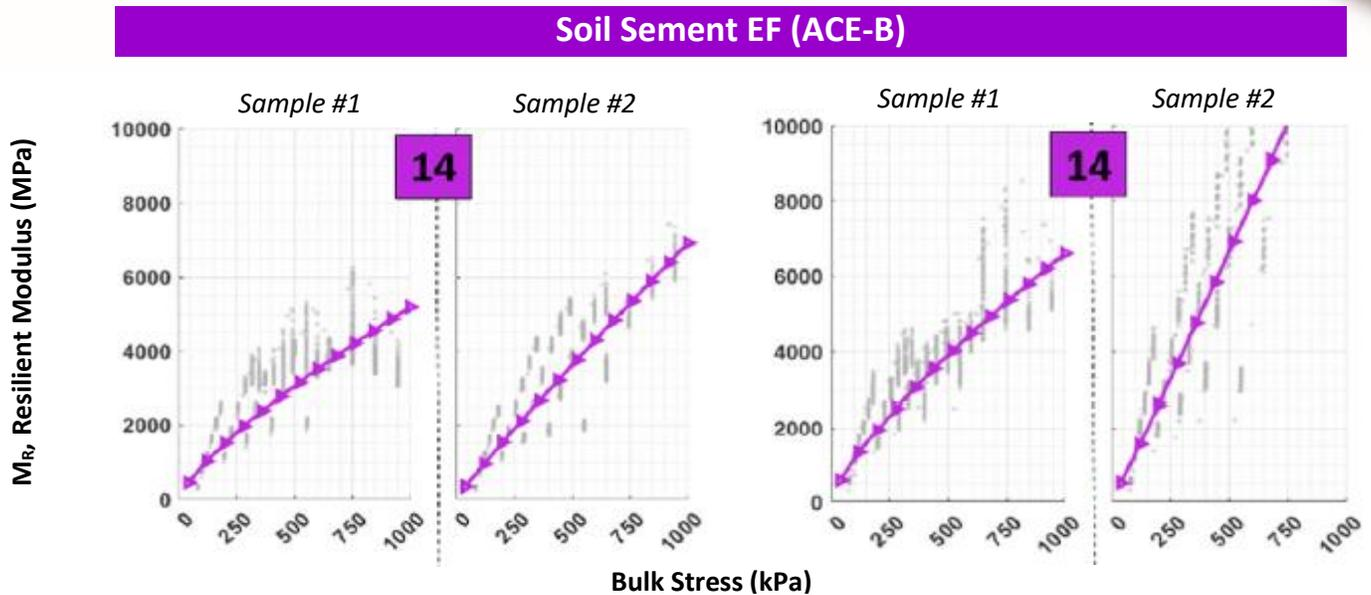
Figure 7: Soil Sement EF (ACE-B) Resilient Modulus ( $M_R$ ) before (left) and after (right) 10 Freeze/Thaw cycles
