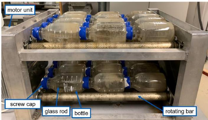
Figure 2: Rolling Bottle Test Setup
