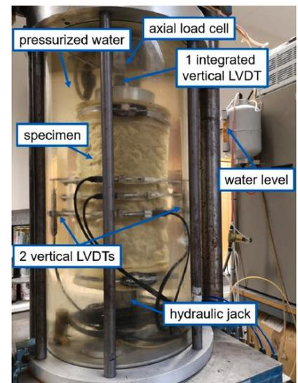
Figure 1: RLTT Specimen Setup
