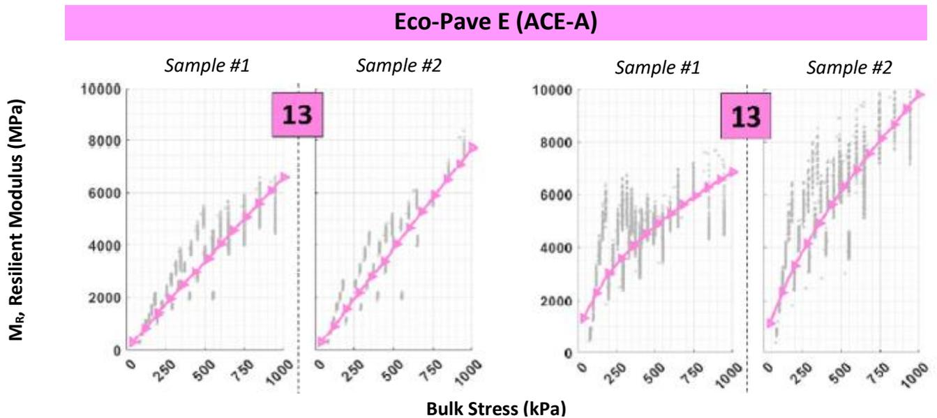
Figure 6: Eco-Pave E (ACE-A) Resilient Modulus ( $M_R$ ) before (left) and after (right) 10 Freeze/Thaw cycles.
