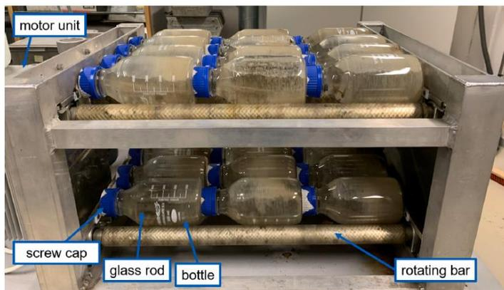
Figure 2: Rolling Bottle Test Setup
