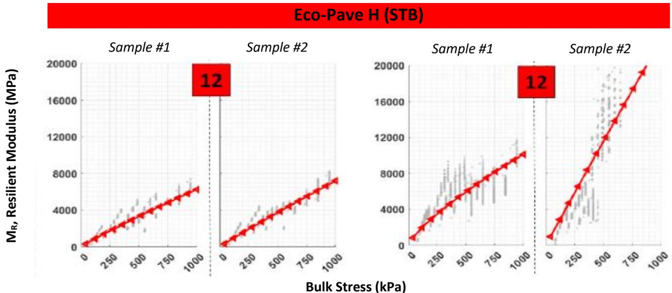
Figure 5: Eco-Pave H (STB) Resilient Modulus ( $M_R$ ) before (left) and after (right) 10 Freeze/Thaw cycles.
